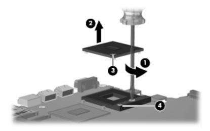
Reverse this procedure to install the processor.
